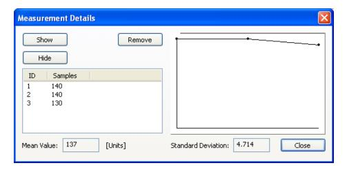
It is possible to delete a measured value if it seems incorrect. Simply select it and click on the *Remove* button. Use the buttons *Show* and *Hide* to show or hide the measurements on the image.
