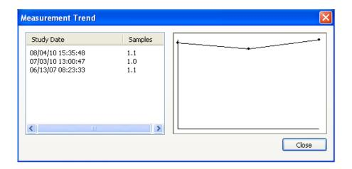
Another useful function is the ability to immediately display the ECG trace from which the measurement was taken. From the measurement menu, when clicking on the *Go to measurement time* option, the software automatically selects the trace on which the measurement was performed.
